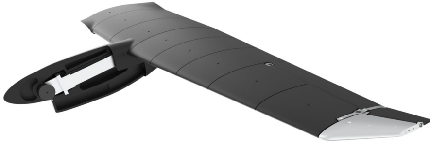
Figure 16: The final assembled wing with an internal view of the nacelle and the IWT installed
